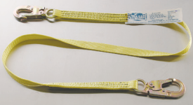
Positioning nylon web lanyard w/ double locking snaps on ends 5,000lbs MBL
