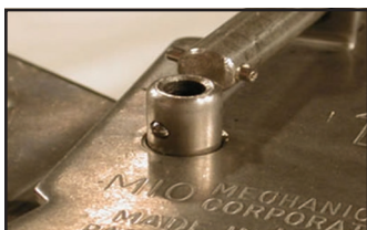
5. Make sure that locking pin balls appear on outside of main assembly.
