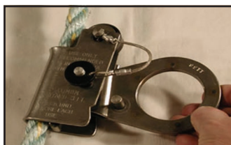
6. Check locking action by pulling down on rope grab handle.
