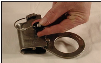
1. Depress the button on the safety locking pin and remove from main assembly.
