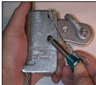
4. Close assembly, align holes and reinsert safety locking pin.
