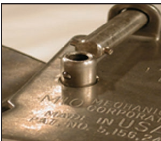
5. Make sure that locking pin balls appear on outside of main assembly.
