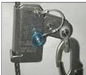
6. Check locking action by pulling down on rope grab handle.
