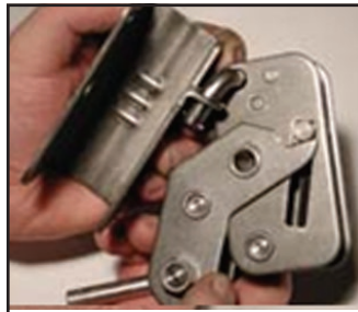
2. Swing cam and level-assembly up and open.
