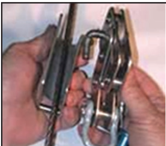
3. Place rope grab on rope with direction arrow pointing up.
