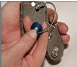
1. Depress the button on the safety locking pin and remove from main assembly.
